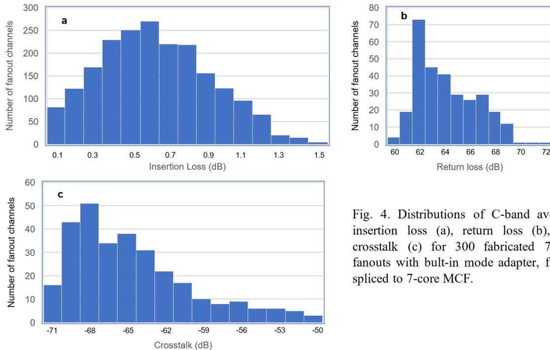
Fig. 4. Distributions of C-band average insertion loss (a), return loss (b), and crosstalk (c) for 300 fabricated 7-core fanouts with built-in mode adapter, fusion spliced to 7-core MCF.
