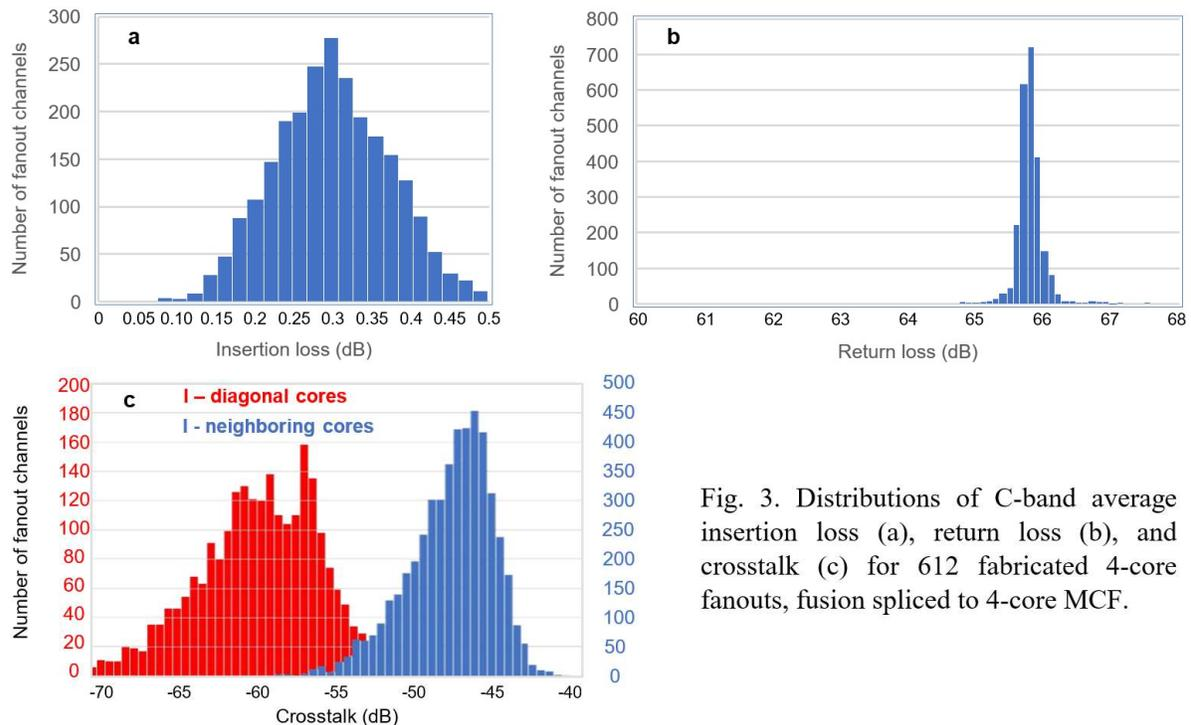
Fig. 3. Distributions of C-band average insertion loss (a), return loss (b), and crosstalk (c) for 612 fabricated 4-core fanouts, fusion spliced to 4-core MCF.
